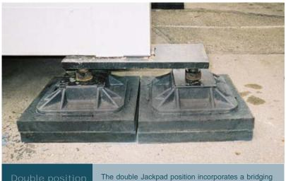
Proof tested 120kN SWL 96kN adjuster and can support a SWL of 96kN. Typically the double adjuster would be used in single storey back to back and double storey single column positions.
