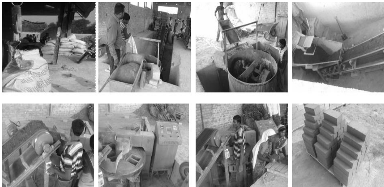
Figure 3: SBA-QD-L brick manufacturing at automated brick plant
