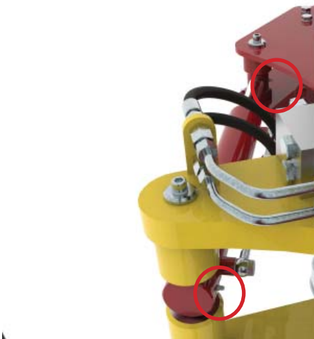
Grab cylinders have one grease nipple in each end (4 total)
