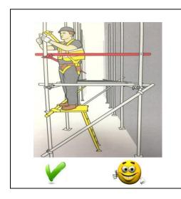
Using either a dummy lift or proprietary scaff steps the scaffolders will erect an advanced guardrail
