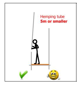
The maximum length of a tube being joined to a hemp **must not** be greater than 5m (16')
