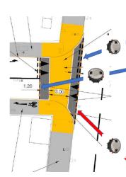
The Junction layout will consist of a <u>string of IRS2 amber bi-directional studs</u> within the road marking arrangement for each junction and be <u>sited facing the cyclist on</u> the path and the drivers on the main carriageway.
