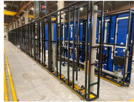
Site fixing brackets utilised to fix to CHtM Track System
