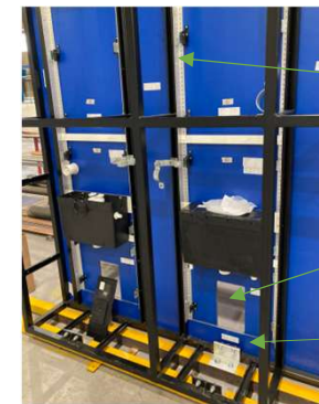
Site fixing brackets utilised to fix to CHtM Track System
