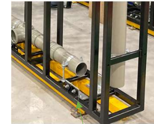
Site fixing brackets utilised to fix to CHtM Track System
