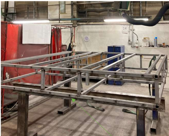
M12 Positive Connection Points fabricated within top of each MIPS frame.
